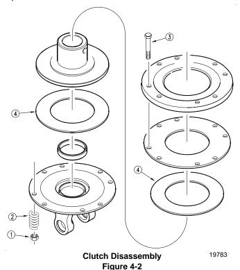
The original friction disc thickness is 1/8" (3.2mm) and should be replaced if the thickness falls below 3/64" (1.1mm). If the clutches have been slipped to the point of "smoking", the friction discs may be damaged and should be replaced. Heat build-up may also affect the yoke joints.
